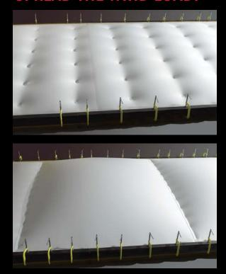
The RhinoBond System spreads the wind load evenly across the roof (top) as opposed to the traditional in-seam fastening method (bottom).
